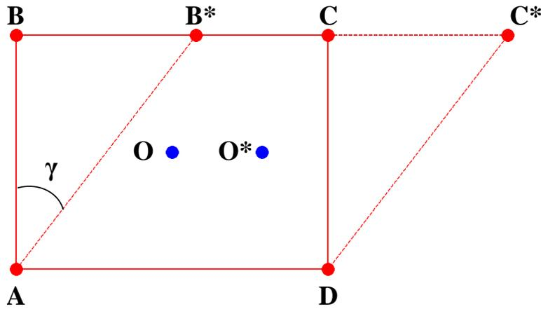
Fig. 3. Sketch of shear transformation.
