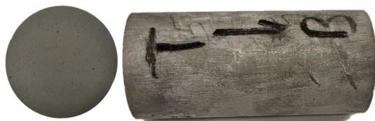
Fig. 4. Graphite core with graphite concentrated at one end (bottom).
